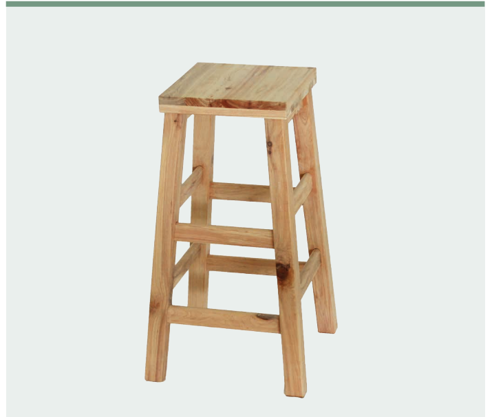
Stool #CH07-0 Classic bar stool in Australian Cypress. Mortice and tenon construction. Very strong and durable. Dimensions: 710 x 400 x 400 mm Species: Australian Cypress
